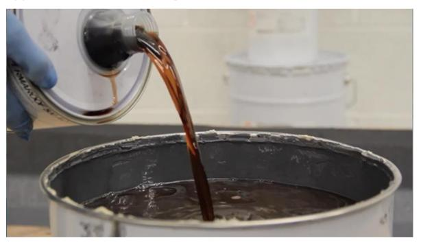
After mixing the accelerator, following the same process as aforementioned for flat surfaces, add the Permathix - usually 250ml of Permathix per 25kg drum is sufficient.
